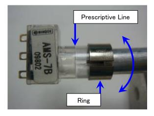
In order to prevent disconnection, a ring is attached to the connecting part of the micro-switch. Depending on the ring size, a little insertion force may be required.
