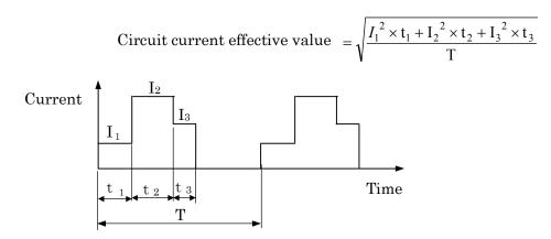
If one cycle (T) is less than 100msec, the rated current of a fuse will be determined by using the reduction coefficient in 2.2 Regular current.
