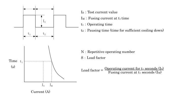
The durability in load factor can be estimated for the following fuses.
